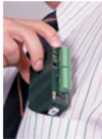
Panasonic Electric Works established a new world standard "SLIM" PLC. Starting from 10 I/O to 32 I/O, the CPU is only 25(w) x 90(h) x 70(d)mm. This is about 1/4 the size of the traditional bulky PLC style called "Brick". The FP0 saves precious panel space and money. Relay output types have removable screw terminal blocks. The power supply connector is also quick to disconnect. Easy installation... especially when duplicating many systems.
